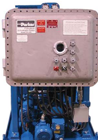
NEMA 7 Explosion Proof
