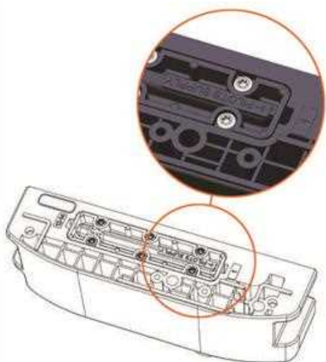
Phase 1. Position of plate for internal air supply
