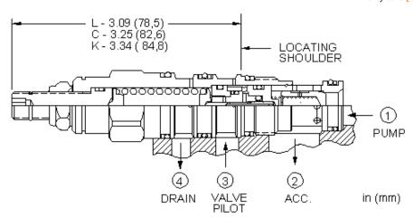
The accumulator sense, pump unload pilot valve is used to sense pressure in an accumulator at port 2 of the valve and when the pressure at port 2 reaches the valve setting, port 3 connects to port 4 to vent a relief valve and unload the pump. This valve has a 15% ratio between unload setting and reset; when pressure at port 2 falls below 85% of the valve setting, port 3 is blocked from port 4 and the pump will come back online to recharge the accumulator.
