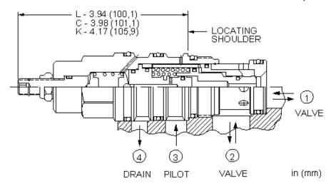
This is a normally closed, balanced poppet, switching element. When pilot pressure is applied to port 3, the poppet remains closed until the pilot pressure reaches the setting established by the integral pilot relief stage, at which point the poppet shifts to the open position.
