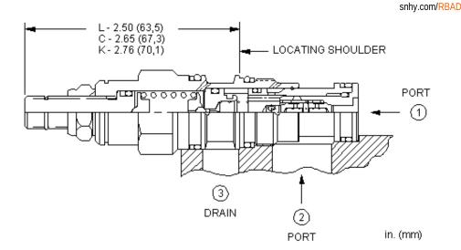
This direct-acting, pilot relief cartridge incorporates back-to-back check valves. This allows it to remotely control 2 other pilot-operated valves or act as a thermal relief for both ends of an actuator. Because capacity is limited to pilot flow, this valve should be used with other valves with comparable pilot flows.
