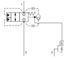
T-SA Cavity Accepts Sun's 2 port Pilot Control Cartridges Pilot Control Cartridge Sold Separately ILOT VALVE
