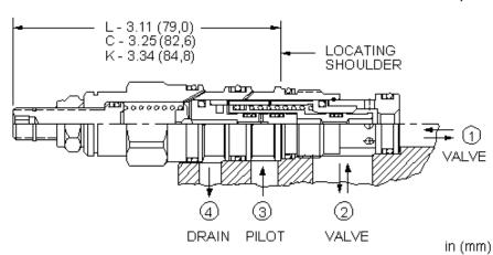
This is a normally open, balanced poppet, switching element. When pilot pressure is applied to port 3, the poppet remains open until the pilot pressure reaches the setting established by the integral pilot relief stage, at which point the poppet shifts to the closed position.
