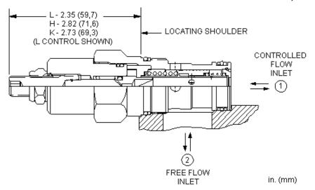
Fully adjustable, pressure-compensated flow controls with reverse-flow check provide precise flow regulation for meter-in or meter-out applications where there may be wide pressure fluctuations. They are infinitely adjustable from nearly closed up to the maximum flow. An integral high-capacity check valve provides unrestricted flow from port 2 to port 1.
