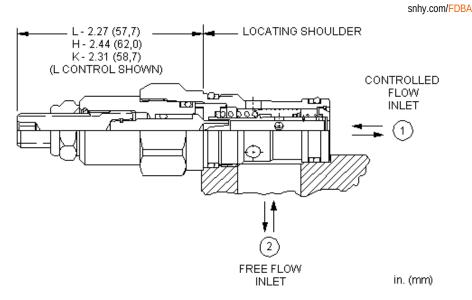
Fully adjustable, pressure-compensated flow controls with reverse-flow check provide precise flow regulation for meter-in or meter-out applications where there may be wide pressure fluctuations. They are infinitely adjustable from nearly closed up to the maximum flow. An integral high-capacity check valve provides unrestricted flow from port 2 to port 1.
