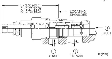
Three-port normally closed modulating elements with relief provide two functions when combined with an external orifice. The mainstage is a bypass compensator that controls a priority flow into the circuit, determined by the external orifice. Input flow in excess of the priority flow is bypassed to tank (port 2). If the inlet (port 1) pressure rises to the valve setting, the valve operates as a normal relief valve.
