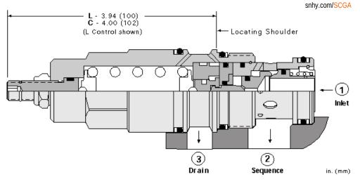
Direct-acting sequence valves with reverse-flow check will supply a secondary circuit with flow once the pressure at the inlet (port 1) has exceeded the valve setting. Additionally, these valves incorporate an integral check valve to provide reverse flow from port 2 (sequence) to port 1 (inlet). The pressure setting of a sequence valve controls the pressure at port 1 relative to the pressure at the drain (port 3).
